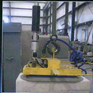
Refractory application: VDF pump pick and place operation
