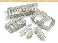
Enidine Wire Rope Isolators protect valuable equipment by combating the harmful effects of shock and vibration. Their rugged all-metal design provides unsurpassed multi-axis isolation, requires no maintenance and is especially suited for harsh environments. Performance is unaffected by chemicals, oils, ozone, abrasives and temperature extremes. The smaller wire rope isolator series utilizes a special patented crimping process, making them especially reliable and cost-effective.
